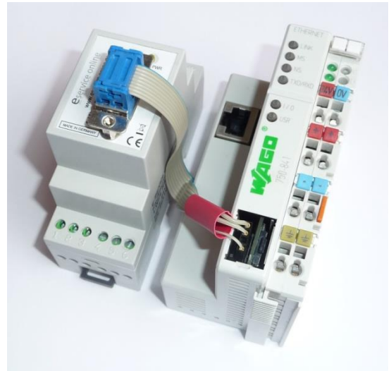
Bild: Systemmontage 1-Wire Buskoppler – SPS
